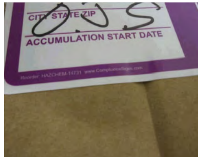
Audit: Accumulation start date missing on spent lamp containers.
